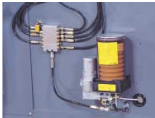
Externally mounted pump for the automatic grease supply system
