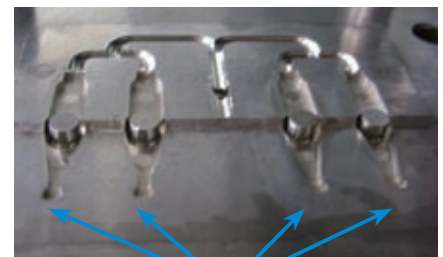
Gas burning is avoided because gas is released from entire parting surfaces.
